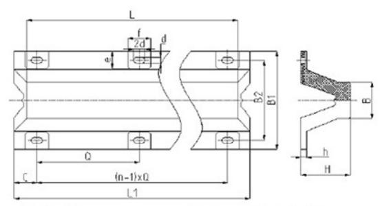
B: Top width of fender; e: Washer mounting hole width;
